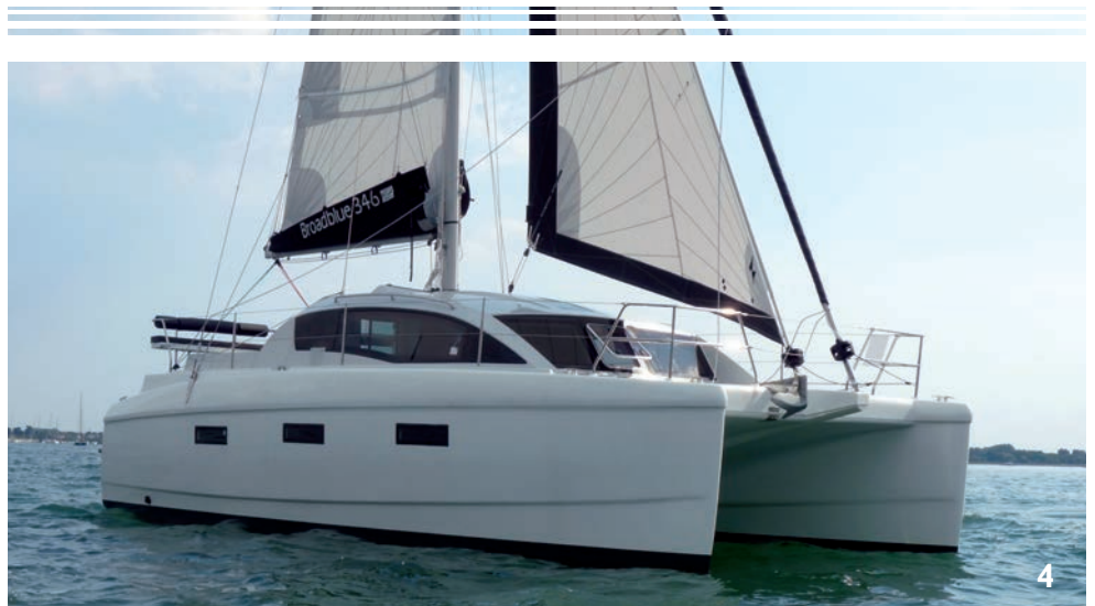
1: A performance rig: mast pre-bend thanks to twin diamond stays on single spreaders, and a generous roach on the mainsail 2: Upwind work is made easy with the self-tacking jib 3: Good bridgedeck clearance, especially forward. Narrow waterline beam 4: The shape of the coachroof and the curved chine smooth the overall lines
